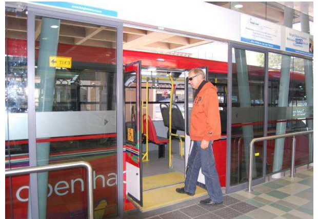
Figure 11. Speedy level boarding onto trunk vehicles.
